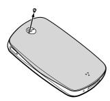
3 Slide the back over of the player down, and then lift up, as shown by the arrow below.
